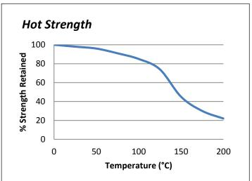
"Hot strength" shear strength tests performed on mild steel. Fully cured then conditioned to pull temperature for 30 minutes before testing. ES5562 can withstand higher temperatures for brief periods (such as for paint baking and wave soldering processes) providing the joint is not unduly stressed. The minimum temperature the cured adhesive can be exposed to is -40°C (-40°F) depending on the materials being bonded.
