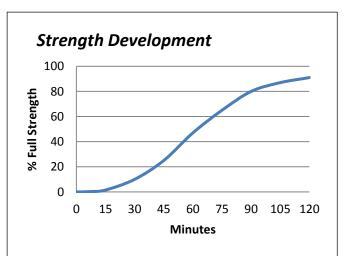
Graph shows typical strength development of bonded components at 23°C. Curing at higher or lower temperatures may affect cure speed.
