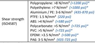
\*Substrate failure was observed.
