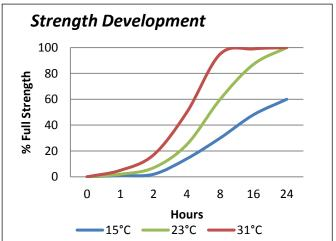
Graph shows typical strength development of bonded components. An increase of 8°C in temperature will halve the cure time. Lower temperatures will result in a slower cure time.
