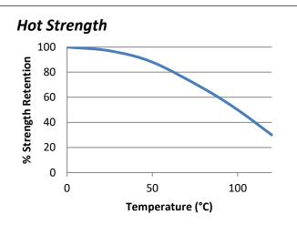
"Hot strength" shear strength. Fully cured specimens conditioned to pull temperature for 30 minutes before testing at temperature.
