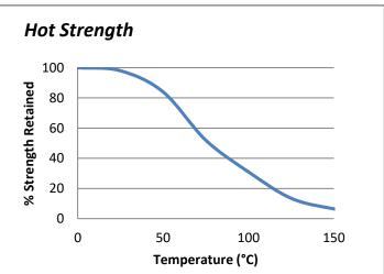
"Hot strength" shear strength tests performed on mild steel. Fully cured specimens conditioned to pull temperature for 30 minutes before testing at temperature. TA4230 can withstand higher temperatures for brief periods (such as for paint baking and wave soldering processes) providing the joint is not unduly stressed. The minimum temperature the cured adhesive can be exposed to is -40°C (-40°F) depending on the materials being bonded.
